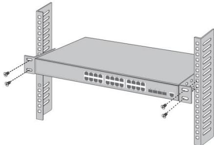
3. Place the switch in the proper position in the rack and support it by the bracket. Fix the L-bracket to the guide groove fixed at both ends of the rack with screws to ensure that the switch is installed on the rack stably and horizontally.
